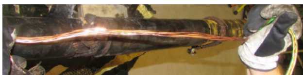
Fig. 5: Investigation of joint failure of EstLink 2
