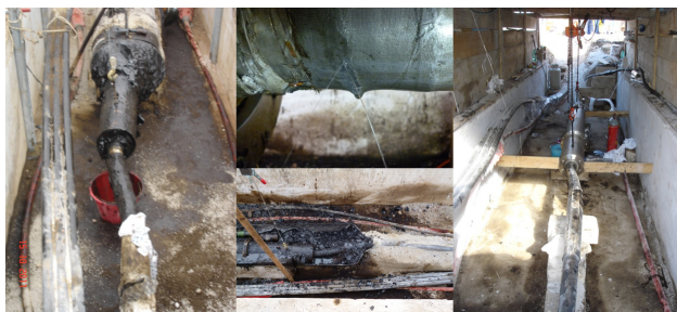
Fig. 4: Damage in joint failure of GRITA
