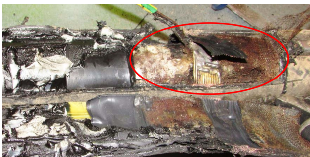
Fig. 6: Moisture damage in EstLink 2 joint failure
